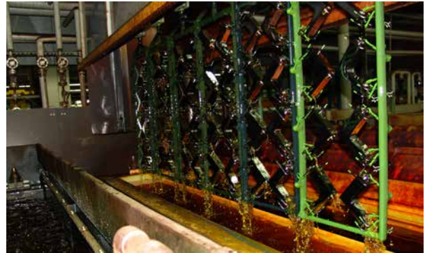
Compared to the old galvanization compound in Schiltach's production facility, the optimized galvanization compound in Offenburg's production facility has a 20% greater production output at the same rate of water consumption
