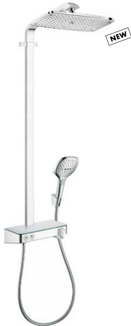
Raindance® Select E 360 ST Showerpipe with Raindance E 360 1jet overhead shower (17 l/min), Raindance Select E 120 3jet hand shower (16 l/min) and ShowerTablet Select 300 thermostat, shower arm 380 mm # 27288, -000, -400 # 27287, -000, -400 (9 l/min) EcoSmart
