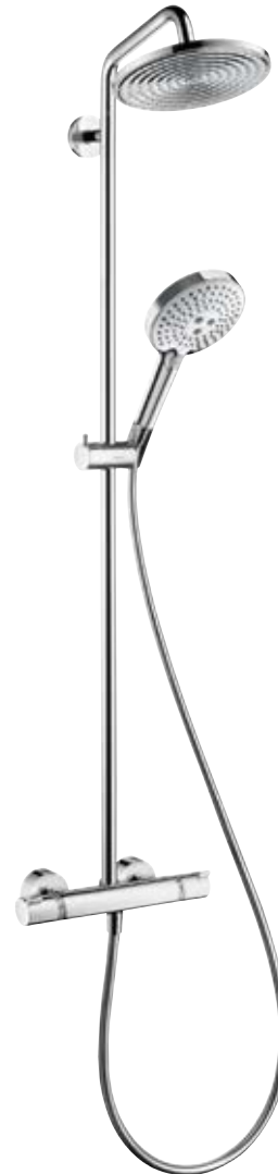
Raindance® Select S 240 1jet Showerpipe with swivelling Raindance S 240 1jet overhead shower (17 l/min), Raindance Select S 120 3jet hand shower (16 l/min) and Ecostat Comfort thermostat, shower arm 460 mm # 27115, -000 Height of the Showerpipe can be reduced
