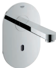
36 273 000 Infrared basin faucet (230 V) wall-mounted, without mixing device projection: 172 mm Chrome spout and escutcheon for concealed box 36 336 000 or 36 337 000
