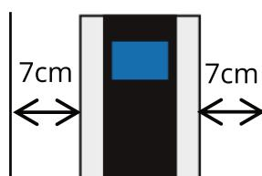
**⚠** When installing several devices side by side, a minimum distance of 10cm must be observed!
