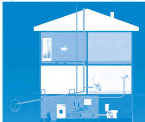
Figure 1: Example of installation with submersible pump:
