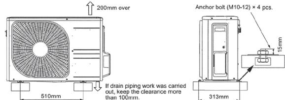
If drain piping work was carried out, keep the clearance more than 100mm.
