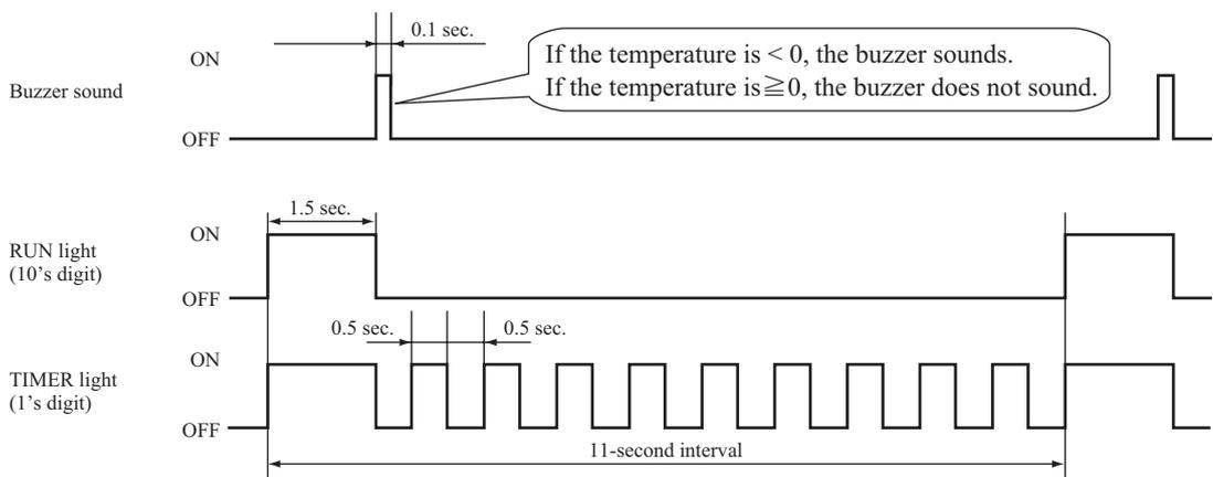
(ii) Discharge pipe temperature sensor
