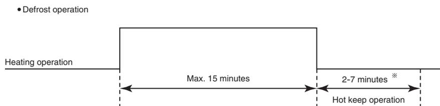
※Depends on an operation condition, the time can be longer than 7 minutes.
