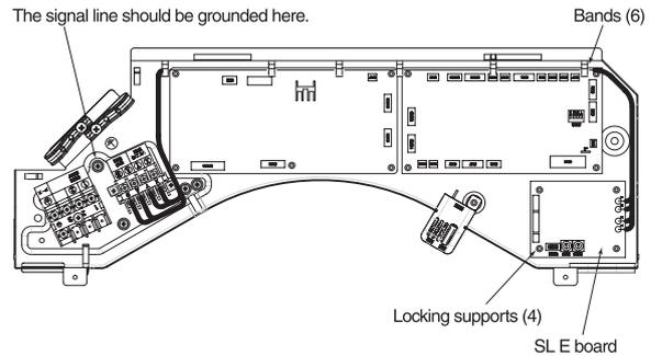
Electrical shock hazard make sure to turn the power off for servicing. Be cautious so that no abnormal force should be applied to the wiring. Do not let the SL E board hung by the wiring. Do not damage the board with a screwdriver.
