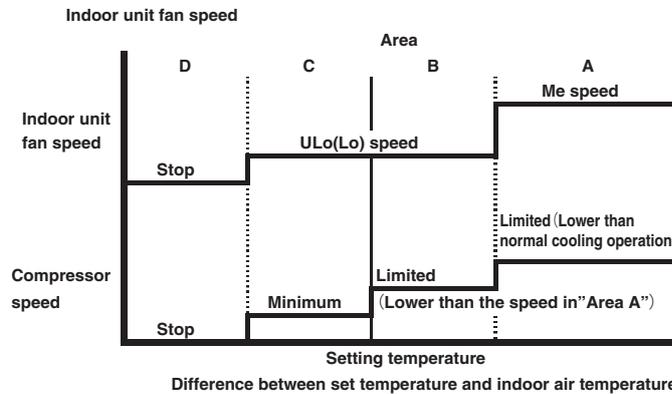
(ii) The indoor unit checks the current area by every 5 minutes, and operates by the next checking.
