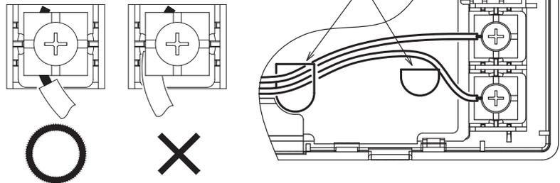
When taking the wiring out from the upper center, open a hole before separating the upper and bottom cases. This will reduce risk of damaging the PCB and facilitate subsequent work.
