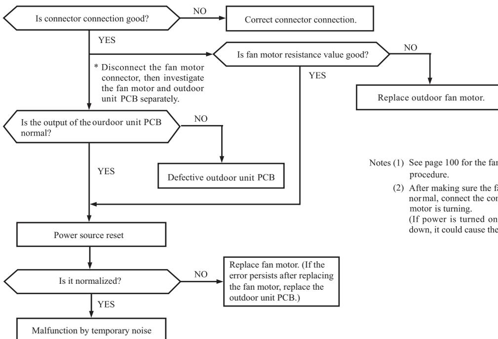
Notes (1) See page 100 for the fan motor and outdoor unit PCB check procedure.
