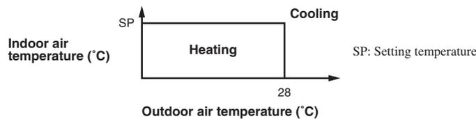
(b) Operation mode is changes when keep cooling and heating thermostat off 20 minutes and be satisfied with following conditions. If the setting temperature is changed with the remote control, the operation mode is judged immediately.
