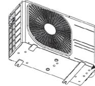
Do not block the drain holes when installing the outdoor unit.
