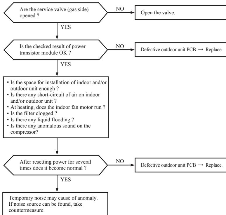
**(8) Phenomenon observed after short-circuit, wire breakage on sensor**
