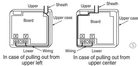
The wiring inside the remote control case should be within 0.3mm<sup>2</sup> (recommended) to 0.5mm<sup>2</sup>.
