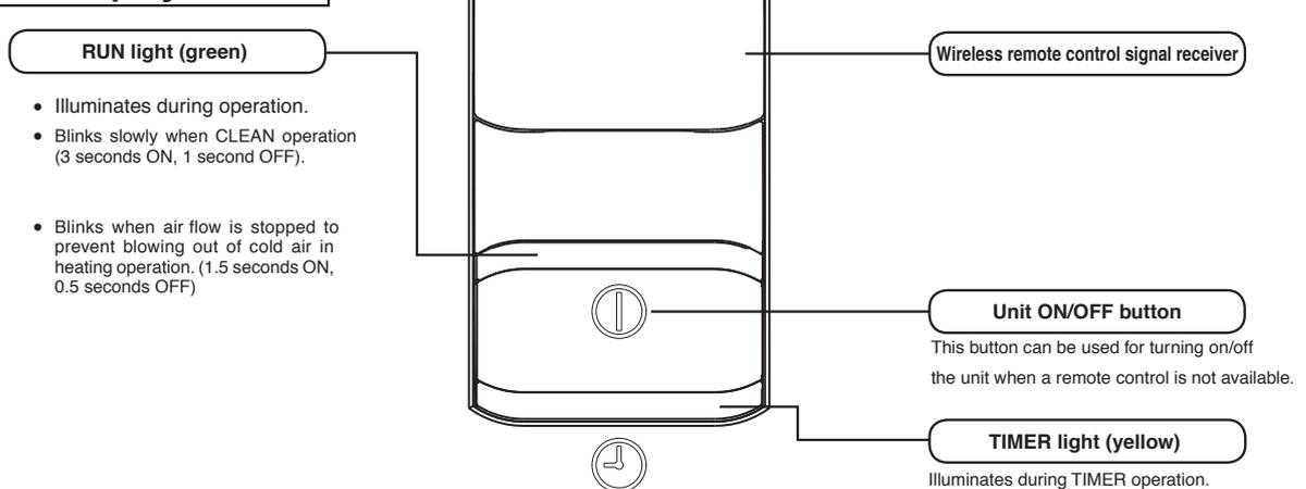
• RUN and TIMER lights blink quickly during invalid operation mode.
