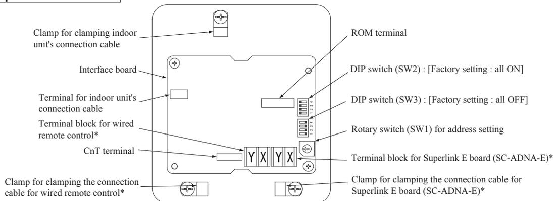
\*Either the connection cables of Superlink E board (SC-ADNA-E) or of wired remote control is connectable.
