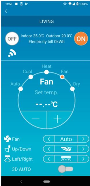
When the operation mode is Fan, Set temp. shows "-".
