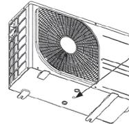
Do not put a grommet on this hole. This is a supplementary drain hole to discharge drain water, when a large amount of it is gathered.
