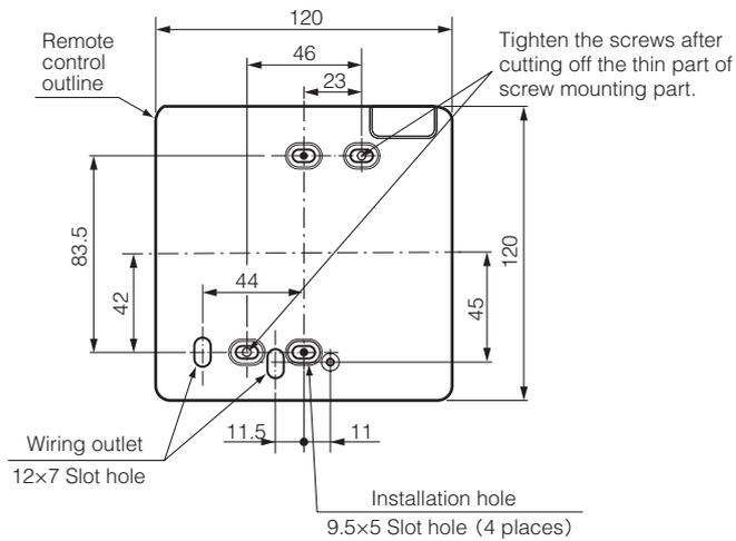
(1) Installation screw for remote control
