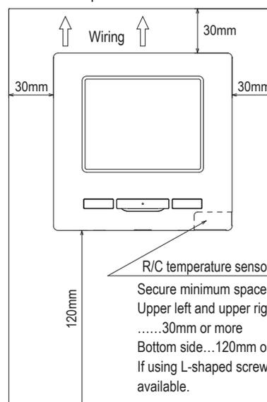
Secure minimum spaces for disassembling the case.
