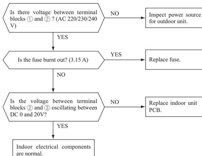
**(b) Indoor fan motor check procedure**
