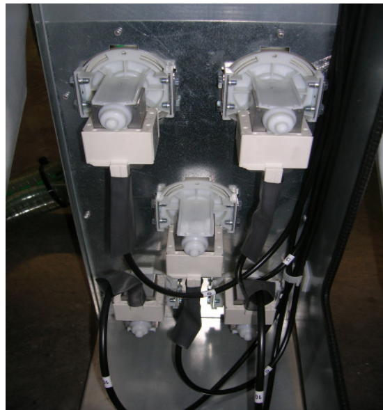
Electrical connection sediment pump
