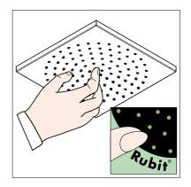
If scale deposits are noticed on the spray face, pour about 3/4" of a commercial scale remover, such as Lime-Away<sup>TM</sup> or CLR<sup>TM</sup>, into a shallow dish. Dilute the remover according to the label instructions.
