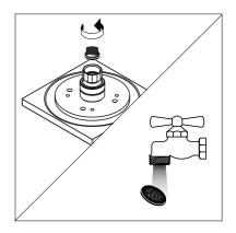
The showerhead incorporates the Rubit<sup>TM</sup> cleaning system. If scale deposits are noticed in the spray channels, turn the water on lightly and rub the spray channels with a finger or a sponge.
