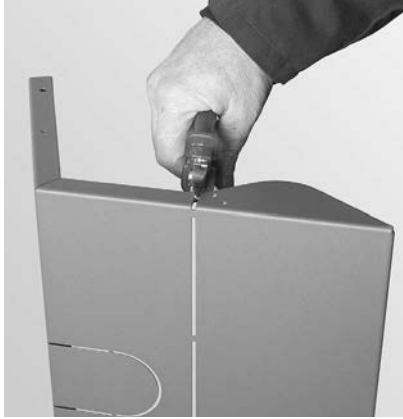
Fig.26 Cut through lever at top and bottom
