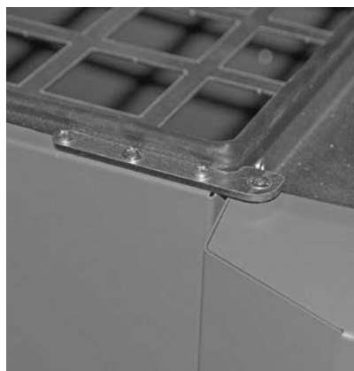
Fig.39 Screw the door hinge and fitted cladding door into position
