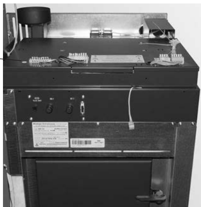
Fig. 24 Open the cover on the control panel
