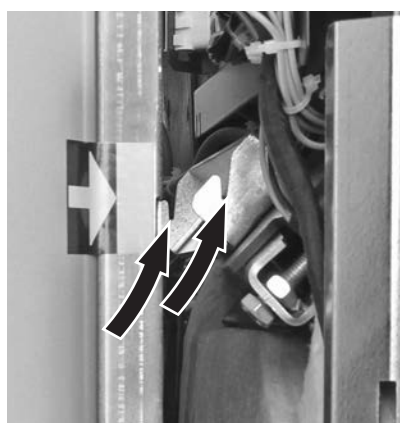
Fig.11 Suspend hopper from 2 hooks, as marked
