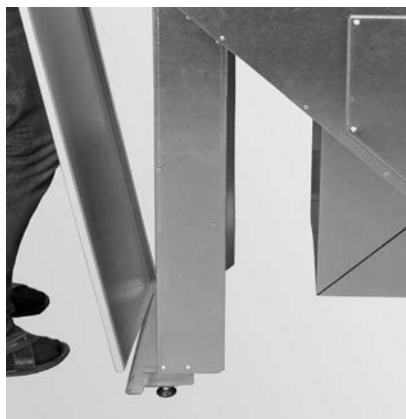
Fig.36 Hook bottom left side panel into position
