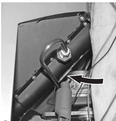
Fig. 15 Insert sensor for safety thermostat auger tube as far as possible
