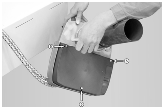
Fig. 2: Removing the intake silencer
